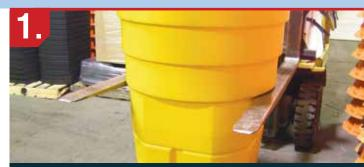
Align the blade with the flat sides of the barrel. If the barrel contains any significant weight, use the center of the blades for balance.
