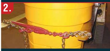
Many forklift blades become loose after years of use. To ensure the blades maintain consistent distance, use a chain binder or a similar type of binder.
