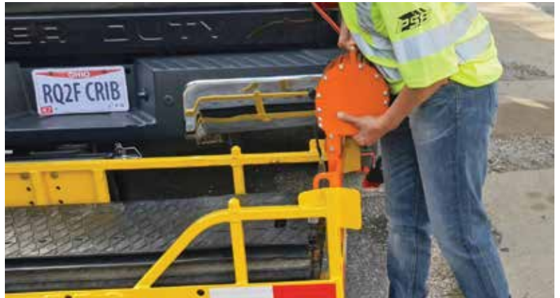
1. Mount Retrieval System to CRIB® Cargo Carrier. Verify that the Retrieval System is fully engaged.
