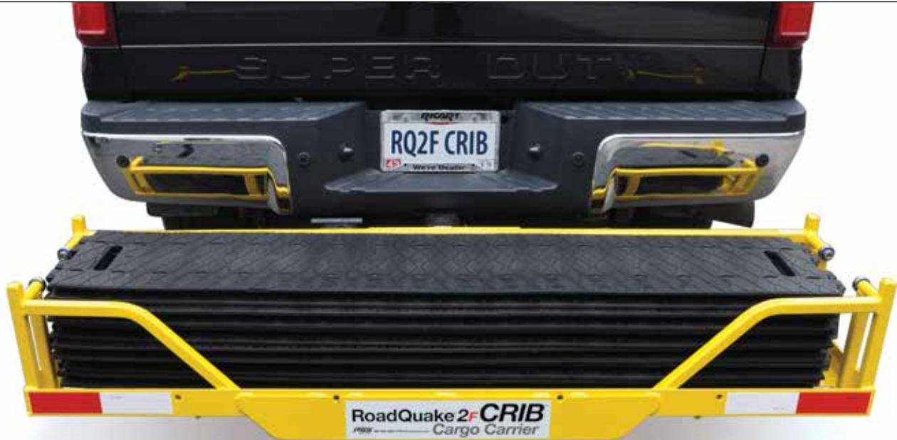
CRIB holds six RoadQuake 2F TPRS. (CRIB Rear Mount shown.)
