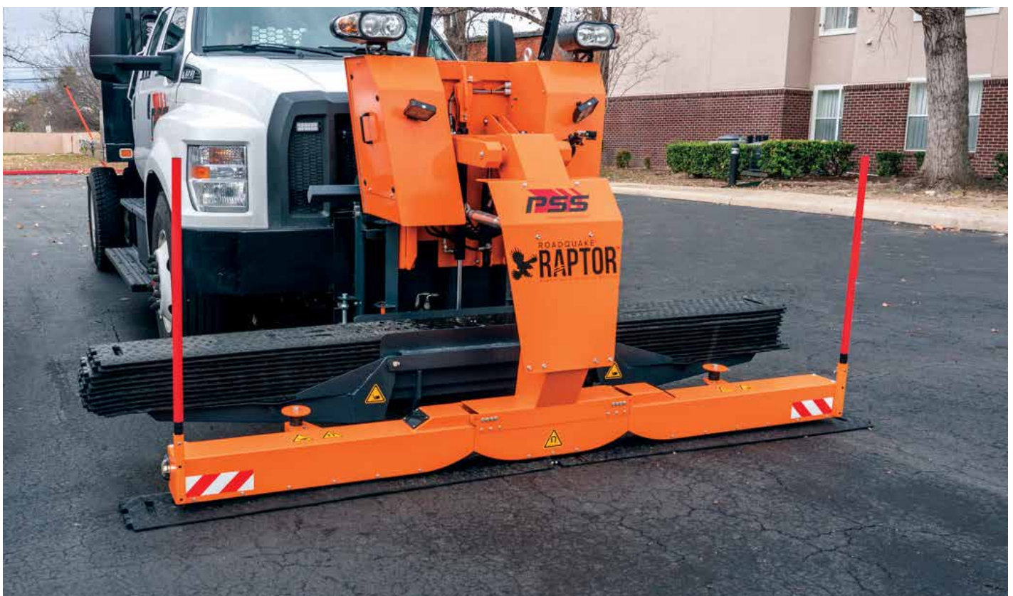
Realignment Operational Mode: RAPTOR straightens misaligned TPRS
