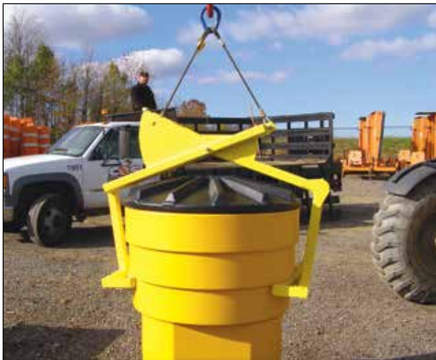
CrashGard Hoist operates with scissor action to clamp and unclamp CrashGard Sand Barrel.
