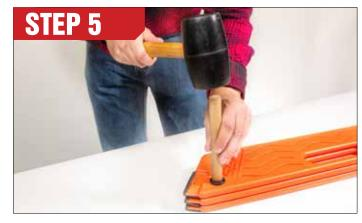
Hit the end of the dowel with the rubber mallet with moderate force. Several strikes may be necessary to completely install the plug. Repeat for all other panels required.
