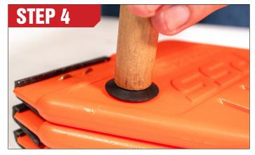
Place the dowel on the top of the plug. Be sure to center the dowel to the plug for even pressure application.
